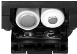
FlexTT5 Battery Polarity
