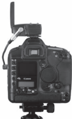
FlexTT5 connected to remote camera
