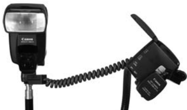
Maximum range, OC-E3 cord with added ferrite clamp
